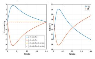
Figure 6: The curves of chromaticity evolution and strength of compensate sextupole.
