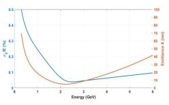
Figure 7: Emittance and energy spread evolution in ramping.
