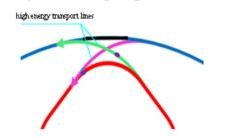
Figure10: The diagram of on-axis swap-out injection.
