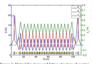
Figure 1: Optical functions and lattice structure of quarter. Table 1: Main Parameters of HEPS Booster Lattice
