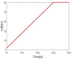
Figure 8: RF voltage during the energy ramp.
