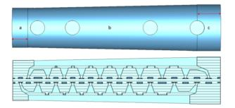
Figure 6: Vacuum area of the cavity(a/c: cylinder, b:cone).
