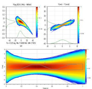
Figure 8: Multi-particle simulation results with 3D field map (left: longitudinal phase space, right: Y-Y' plot, bottom: beam envelop in X, X and Y are the same).
