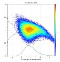
Figure 5: Longitudinal phase space after de-buncher.
