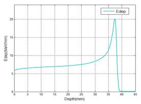
Figure 3: Energy deposition curve of 250MeV proton beam in tungsten.
