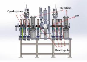
Figure 1: Layout of MEBT of C-ADS Injector II.
