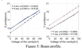
Since the linear coefficient  $R^2$  is 0.9987 in the two directions correspondingly, the measurement result is very close to linearity.
