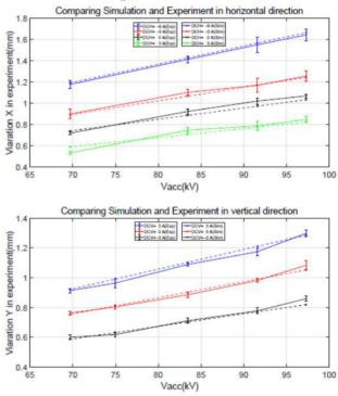
Figure 4: Simulation and experiment comparison.
