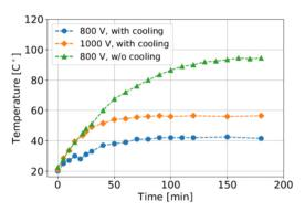
Figure 5: Maximum temperature rising as a function of time with constant gap voltage.
