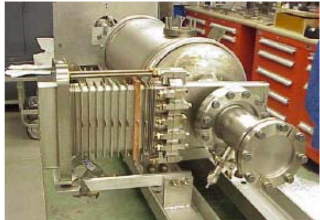
Figure 5. Waveguide coupler for the CEBAF upgrade cavities: a single ceramic window at room temperature replaces the double windows present in the original CEBAF design. The high thermal gradients along the waveguide require a careful design. [15]
