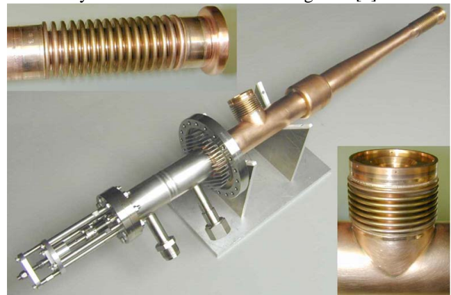
Figure 3. Details of the center conductor of the APT coupler, with the BeCu bellows, which allow the coupling variation (upper left). [8]
