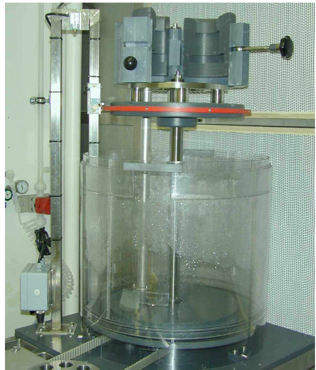
Figure 3: Saclay-type high pressure rinsing system for single-cell cavities. The turn-table (with red ring) is moving up and down on a fixed thread with the nozzle on its top. The cavity is fixed by the grey plastic clamps.
