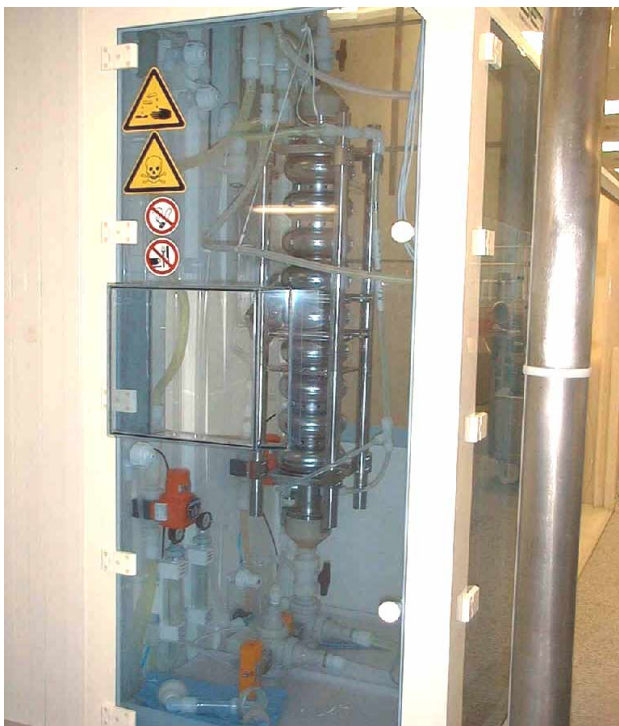
Figure 2: Electropolishing of a single-cell cavity at CERN (upper, by courtesy of CERN) and BCP of a TTF nine-cell cavity at DESY (lower)
