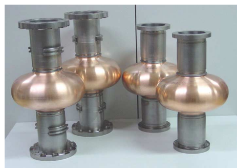
Figure 12: NbCu cavities INC1-INC4 hydroformed from explosive bonded tubes of 4 mm wall thickness. Resonance frequency: INC1-1,3051GHz, INC2-1,3038GHz, INC3-1,3025GHz, INC4-1,3039GHz.
