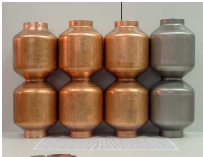
Figure 6: Example of tube necking at the iris area
