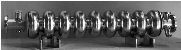
Figure 1: A TESLA niobium 9-cell cavity. The length of a cavity is about 1m.
