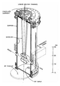
Fig.2 Cutaway view of superconducting quarter wave resonator in the JAERI Tandem-Booster
