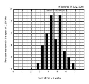
Fig. 5 Histogram of the field gradients at the rf input of 4 watts
