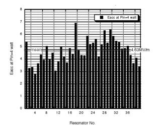
Fig. 4 Field gradients E<sub>acc</sub> at the rf input of 4 watts measured in July 2001
