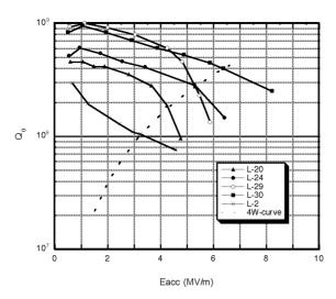
Fig. 6 Typical Q-E<sub>acc</sub> curves
