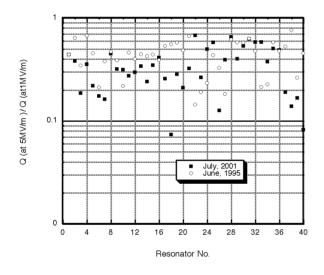
Fig. 7 Ratio of Q at 5 MV/m or near 5 MV/m to Q at 1 MV/m
