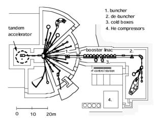
Fig.1 Layout of the JAERI Tandem and its booster
