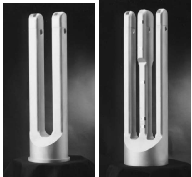
Figure 1: The prototyped resonators: Two Stub Half Wave Resonator (Left) and Three Stub HWR (right).
