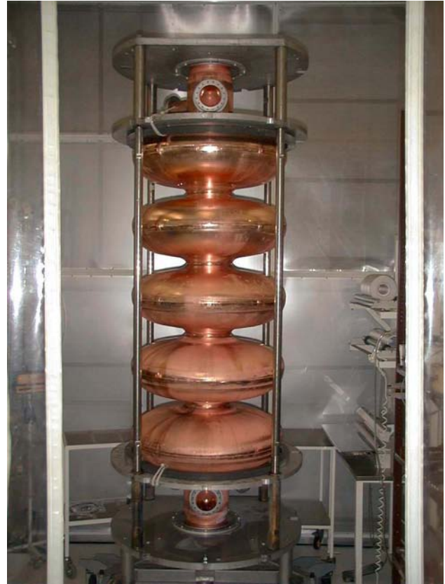
Figure 2, five-cell cavity ready for the sputtering cathode insertion
