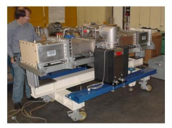
Figure 7: Two 500 MHz RF windows assembled and baked at ACCEL after final leak-check, ready for RF processing at Cornell.
