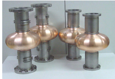
Figure 1: NbCu cavities INC1-INC4 hydroformed from explosion bonded tubes of 4 mm wall thickness. Resonance frequency: INC1-1,3051GHz, INC2-1,3038GHz, INC3-1,3025GHz, INC4-1,3039GHz.
