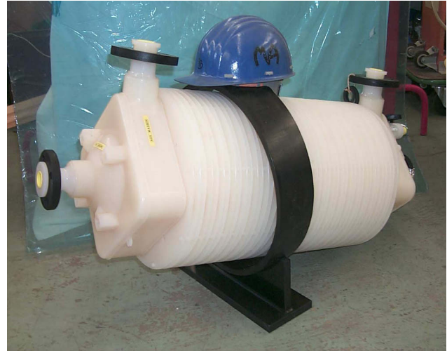
Figure 4: Acid Heat Exchanger
