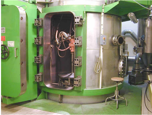
Figure 5: Chamber used for Inert gas Plasma Spraying.
