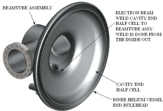
Figure 4. Cavity 1/2 cell welded to beamtube assembly.
