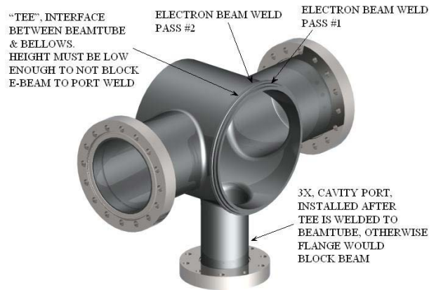
Figure 2. coupler beamtube of the \beta=0.64 cavity.
