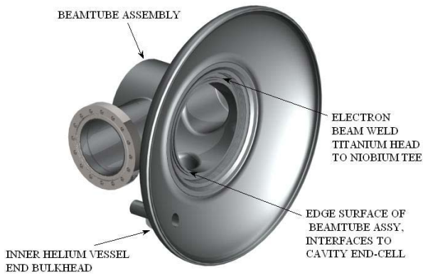
Figure 3. Helium vessel head welded to cavity beamtube.
