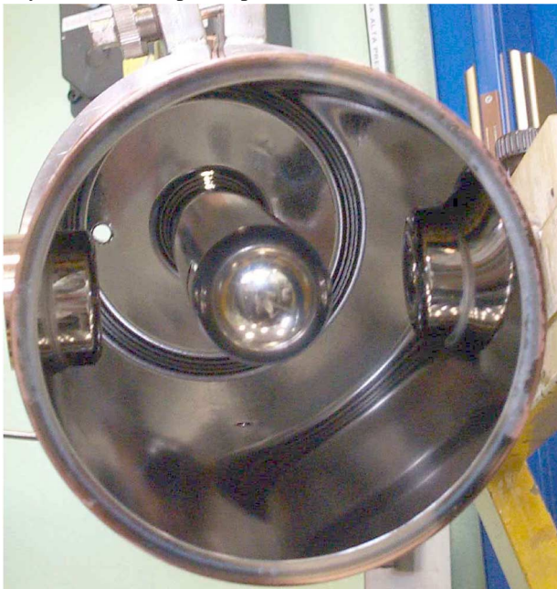
Fig.11: A medium \beta resonator after being stripped by the Pb layer and Nb sputtered. The hole in the shorting plate was used in the Pb electroplating process.
