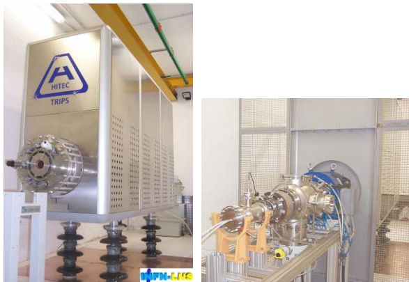
Figure 3. The TRIPS high voltage platform (left) and the first section of the LEBT line.
