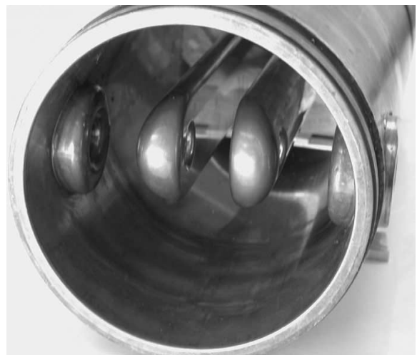
Figure 4: Copper prototype for \beta=0.1 150 MHz HWR2 utilizing two RF demountable joints.
