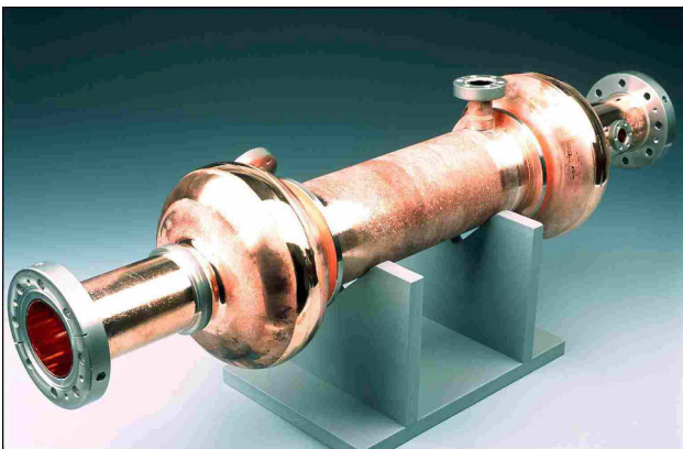
Fig. 5: Prototype of the S3HC cavity built at CERN.
