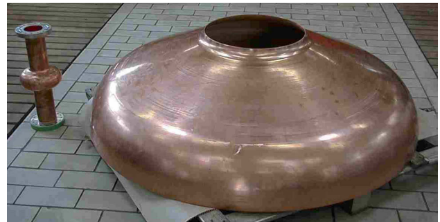
Fig. 6: A 1500 MHz cavity and a 200 MHz half cell.
