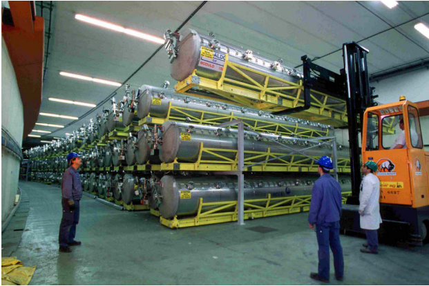
Figure 2: The 72 LEP modules stored in the ISR ring.
