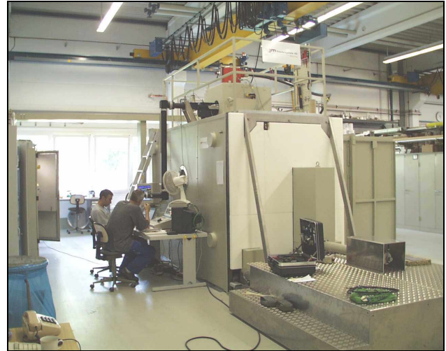
Figure 6: View on the EB welding machine at DESY
