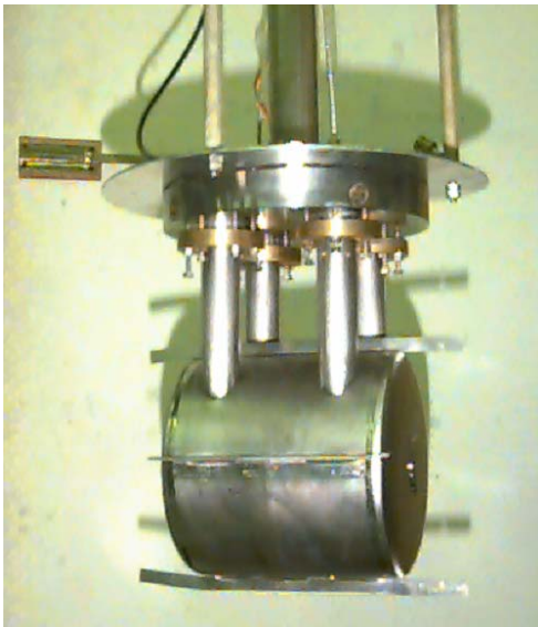
Figure 3. PACO cavity mounted in the test cryostat.
