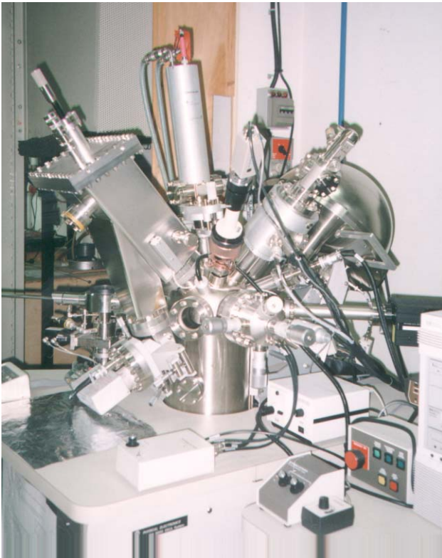
Figure 6, The XPS-Auger apparatus used for the Niobium surface analysis.
