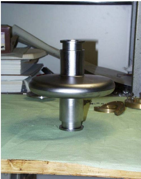
Figure 13. the 1400 MHz test cavity
