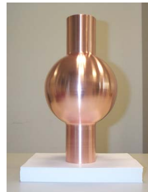
Figure 5. Single cell, seamless, spherical cavity, built at INFN-LNL, to be sputter coated at CERN.
