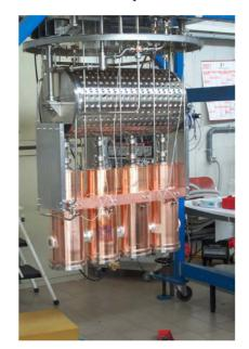
Fig. 1 : 160 MHz, medium  $\beta$  cryostat equipped with four Nb/Cu sputtered resonators
