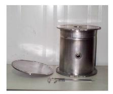
Fig. 8: The 352 MHz quarter wave cavity.
