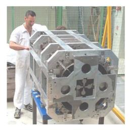
Fig. 3: SRFQ1 during frequency rough tuning test, which precede the final EB welds.
