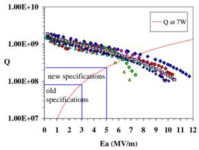
Figure 5: Rf test results of the PIAVE 80 MHz, quarter wave resonators equipped with mechanical dampers. Only cavity n. 8 (square marker) underwent high pressure rinse.
