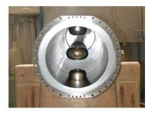
Figure 6: View of a PIAVE type bulk niobium cavity.
