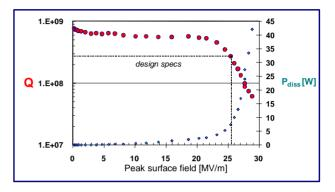
Fig. 4: SRFQ2 rf test results.
