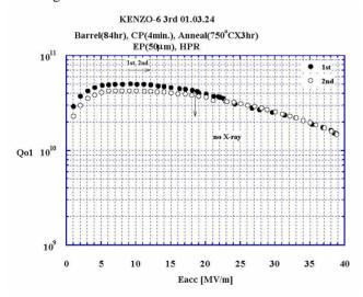
Fig. 10 - The cavity KENZO 6 is a bulk Niobium monocell spun at LNL, and electropolished at KEK.
