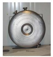
Fig. 7: The TRASCO 352 MHz reentrant cavity prototype.
