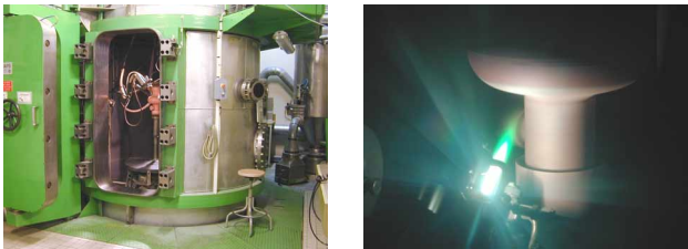
Figure 10: Sealed chamber for IPS and a 1.3 GHz cavity during the deposition process.
