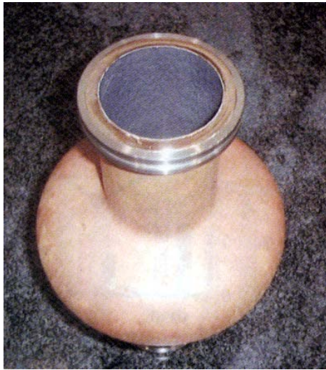
Figure 11: A photo of a Nb/Cu clad seamless sc cavity.
