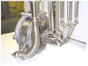
Figure 3: An ANL cavity ( $\beta$ =0.29, 340 MHz, 2-gap) set on the vertical cryostat insert.
