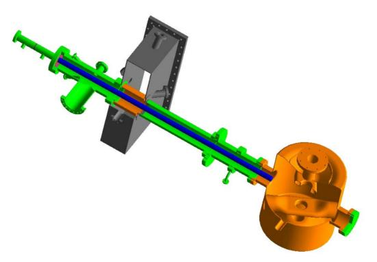
Figure 6: The power coupler being designed for spoke cavities.
