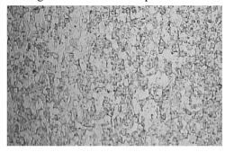
Figure 13. Grain structure of RRR Nb.
