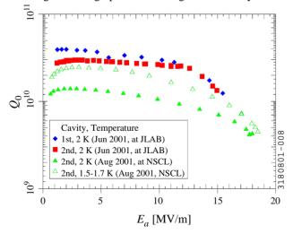
Figure 6. Measured dependence of Q on accelerating gradient for the RIA cavity.
