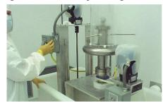
Figure 5. High pressure rinsing of RIA cavity.
