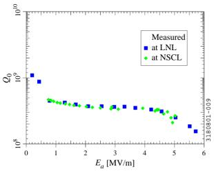
Figure 10. Measured dependence of *Q* on accelerating gradient for 80 MHz cavity, before and after etching at NSCI
