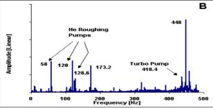
Figure 7. Microphonics spectrum from FFT of (A) cavity's phase lock loop/error signal, and (B) accelerometer on top of Dewar.
