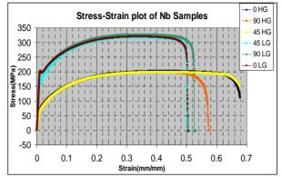
Figure 12. Stress-strain plot of Nb.
