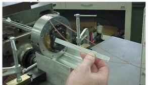
Figure 11. Superconducting quadrupole during magnetic field mapping at room temperature.
