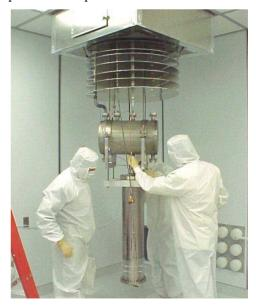
Figure 9. QWR installed on insert.
