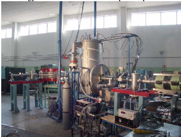
Fig. 3 Layout of proton beam accelerating structure
