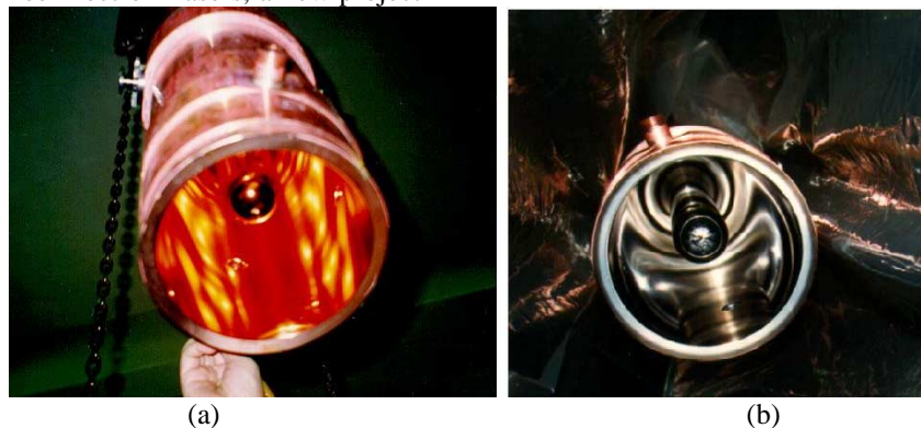
Fig. 1 QWR after electro-polishing (a) and after niobium coating (b)
