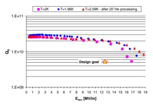
Figure 3: SNS  $\beta$  =0.81 vertical test results.
