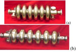
Figure 1: SNS prototype cavities: (a)  $\beta = 0.61$ and (b)  $\beta = 0.81$ .
