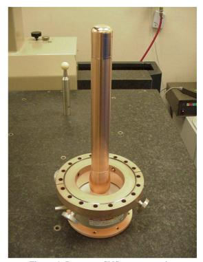
Figure 4: Prototype SNS power coupler.
