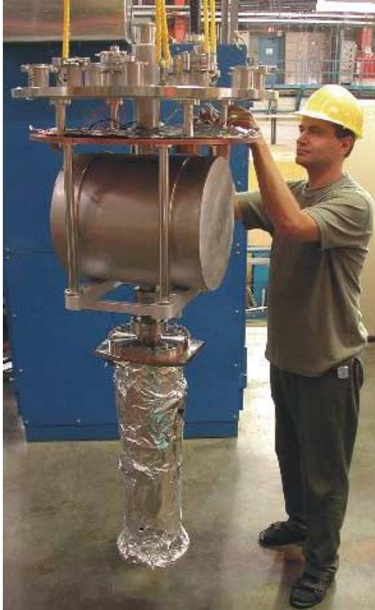
Figure 9: ISAC-II test cryostat inner assembly with ‘dummy’ copper cavity.
