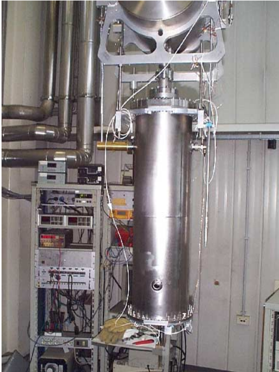
Figure 6: TRIUMF medium beta prototype cavity before cold test at INFN-LNL.
