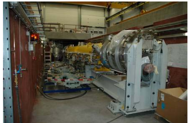
Figure 3: Picture of the cryomodule test bench (CMTB) at DESY.
