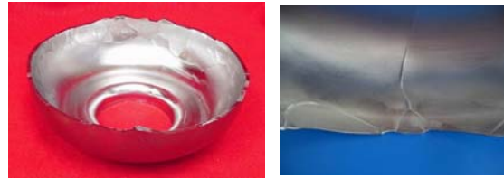
Figure 4: Forming of half cells from sheet, showing “earing” and grain slippage [7, 8].
