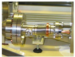
Figure 5: Coupler cold bellows lateral deformation.
