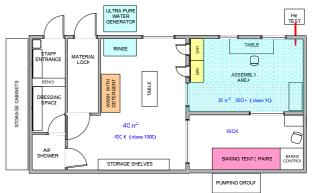
Figure 8: Clean room for assembly and baking for 200 couplers / year.
