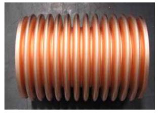
Figure 7: Copper coated bellow for the inner coax conductor.
