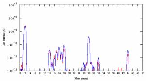
Fig. 9: Typical spectrum recorded by RGA on a pair of couplers after conditioning
