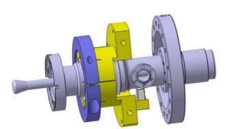
Figure 6: Coupler cold bellow support design proposal, the support is the part of the 4 K thermal shield.
