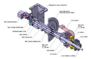
Figure 1: XFEL-type input RF power coupler.
