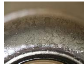
Figure 1: Q_0 vs. E_{acc} measured at 1.44 K at Saclay [9] on a 1.3 GHz single-cell cavity treated by BCP (top) and post-purified at 1400 °C, resulting in a rough surface with pronounced grain boundaries (bottom).
