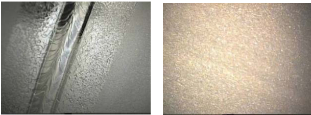
Figure 3: Picture of the inner surface of the equatorial weld before (left) and after (right) removing 60 \mu\text{m} by centrifugal barrel polishing (Courtesy of T. Saeki).
