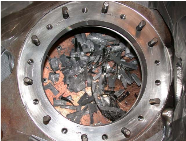
Figure 5: The remains of a turbo pump after touch down failure in cryomodule CM4.
