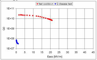
Figure 2: Test result of cavity 1AC9. After a fast cooldown (red dots) the cavity showed good performance and Q values above  $1\cdot 10^{10}$  for accelerating gradients below 18 MV/m. At 22 MV/m the cavity was limited by quench. For a second test the cavity was cooled down very slowly resulting in very low Q values and gradients, indicating that the niobium of the cavity was contaminated with hydrogen (Q disease).
