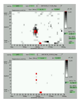
Figure 3: temperature maps taken during (top) and just below the quench (bottom). The maps show the source of the quenc close to the equator. It is not clear if a material defect or multipacting is responsible for the quench.
