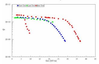
Figure 4: RF test results of cavity 1AC1. First test (blue dots), achieved with standard BCP treatment, Best test (red dots) achieved with standard electro polishing treatment and last test (green dots) achieved with new electro polishing method. During the last test, at 22 MV/m a quench limited the cavity to reach higher fields. Multipacting was observed from 19 MV/m on during that test.
