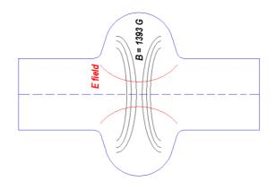
Figure 1: A simple illustration of a 3.9 GHz RF cavity with external dipole magnetic field of 1393 Gauss in the center to form the ECR condition.
