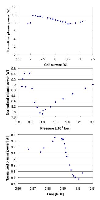
Figure 5. The normalized plasma power absorption at 10 W RF input power; top: Ar pressure  $1.0 \times 10^{-4}$  Torr; middle: Ar pressure  $1.0 \times 10^{-4}$  Torr and Coil current 8.5 A; bottom: Ar pressure  $4.4 \times 10^{-4}$  Torr and coil current 8.6 A
