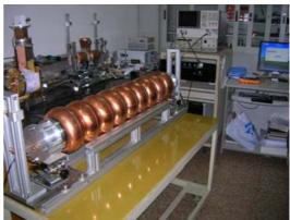
Figure 2: Field flatness measurement system of the ICHIRO cavity.
