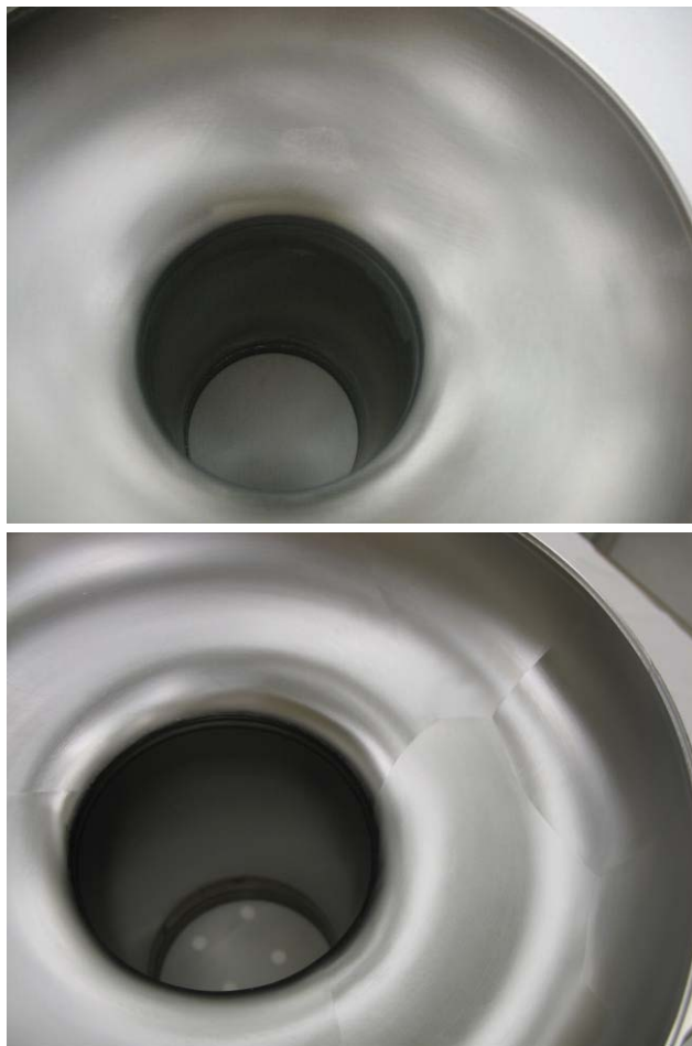
Figure 1. Fine grain (top) and large grain (bottom) half-cells after the iris weld.
