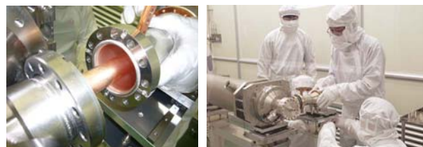
Figure 14: Installation of a cold coupler into a cavity
