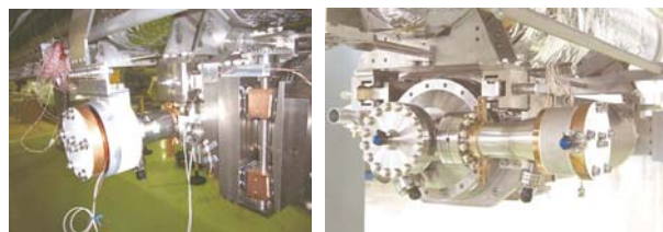
Figure 15: Baking heater and 80 K shielding attached on a cold rf window (Left), and an assembled cavity mounted on 2 K gas return pipe (Right).
