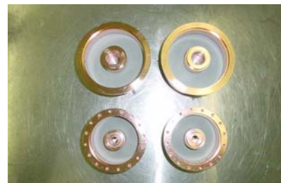
Figure 5: Two warm rf windows (Top) and two cold rf windows (Bottom) after the initial brazing.
