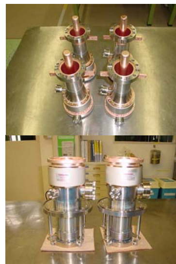
Figure 6: Four cold couplers (Top) and two warm couplers (Bottom) after the final brazing.
