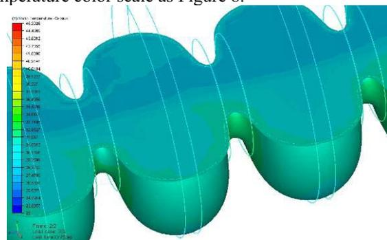
Figure 9. Steady-state temperature in the plane of the electrolyte top surface and at the fluid/cavity interface, with 30°C external water bath boundary conditions.
