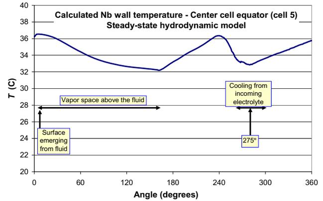
Figure 5. Model temperature variation of the niobium wall at the equator of the center cell.
