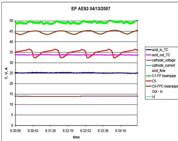
Figure 7. Logged process conditions during EP of cavity AES3 at JLab.
