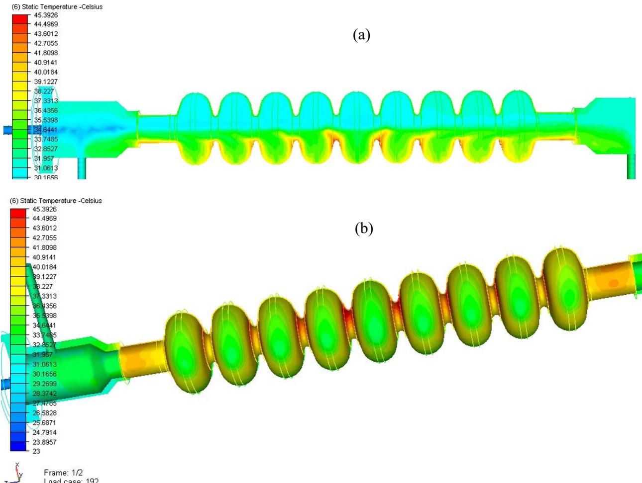
Figure 4. Steady-state solution temperatures at (a) top electrolyte surface and (b) interface with cavity wall.
