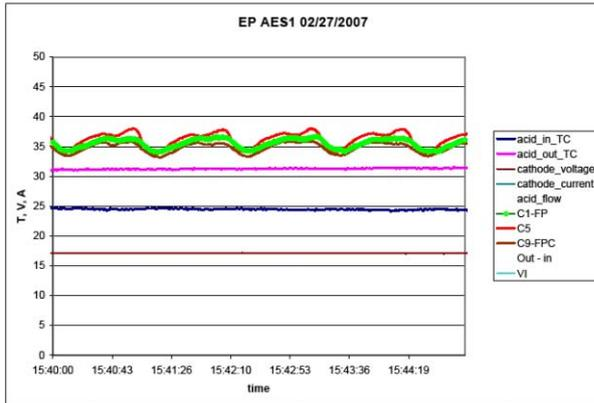
Figure 6. Logged process conditions during EP of cavity AES1 at JLab.
