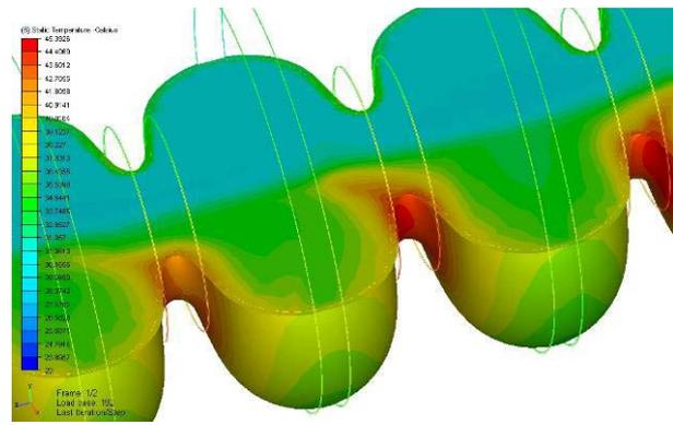
Figure 8. Steady-state temperature in the plane of the electrolyte top surface and at the fluid/cavity interface.
