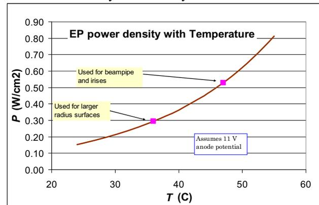
Figure 2. Derived heat flux as a function of local temperature.
