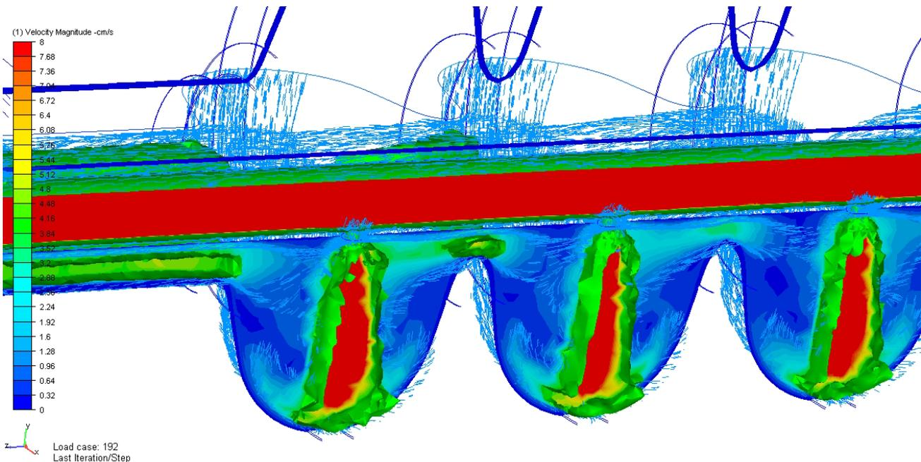
Figure 3. Steady-state electrolyte velocity magnitude in three end cells and beamtube, with 10 lpm total supply flow.
