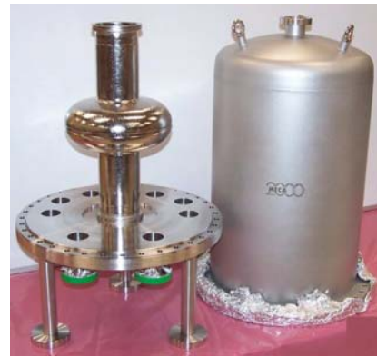
Figure 9: New apparatus for fast baking in oxygen-free atmosphere on open-ended cavity.
