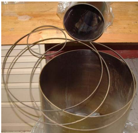
Figure 3: Quarter-wave cavity cylinder and center conductor with “trim rings” produced by wire EDM.
