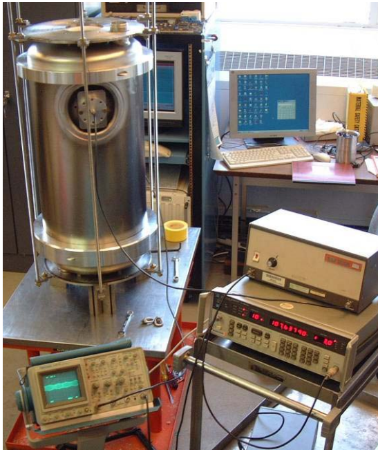
Figure 2: Clamped-up cavity during frequency check.
