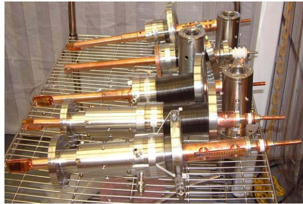
Figure 7: Group of five adjustable loop-type input couplers. The lower two are complete while the upper three have their bellows sections removed to show the antenna. Total coupler stroke is 7.6 cm.
