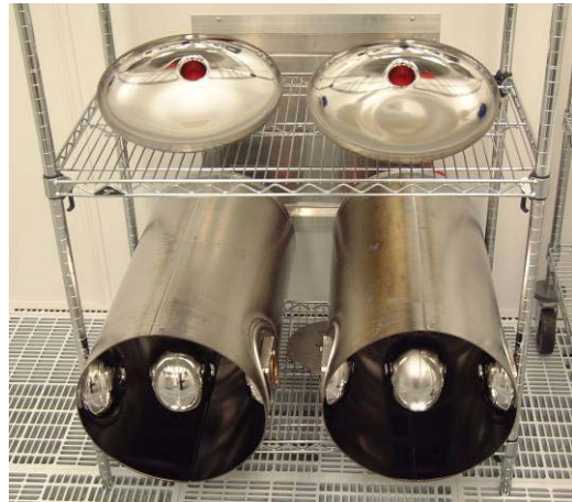
Figure 4: End domes (top) and cylinder/toroid/center conductor assemblies (bottom) following EP.
