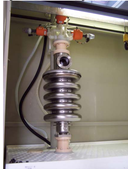
Figure 5: the cavity on the automated BCP station
