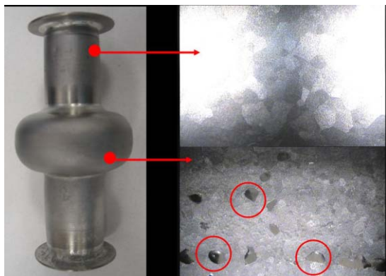
Figure 2: \text{Nb}_3\text{Sn} 6GHz cavity obtained using the “ hybrid process ”. The unreacted Sn problem is still present.
