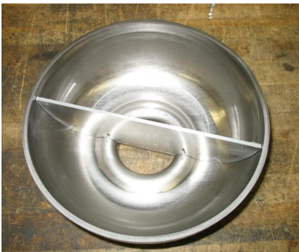
Figure 2: Reentrant half-cell with checking fixture.
