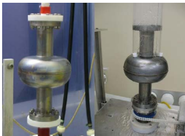
Figure 5: A half-reentrant cavity is shown during an interior etch on the left and during a high-pressure rinse (HPR) on the right.
