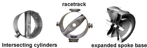
Figure 4: A simple spoke cavity based on intersecting cylinders (left). A “racetrack” design (middle) to minimize E_{PEAK} and an optimized spoke (right) to minimize B_{PEAK} .
