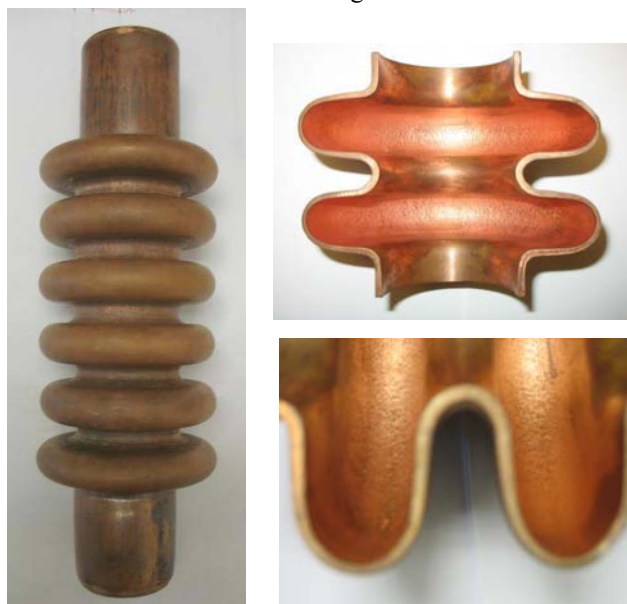
Figure 5: Samples of hydroformed copper cavities.
