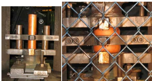
Figure 4: Industrial hydroforming of copper tubes.
