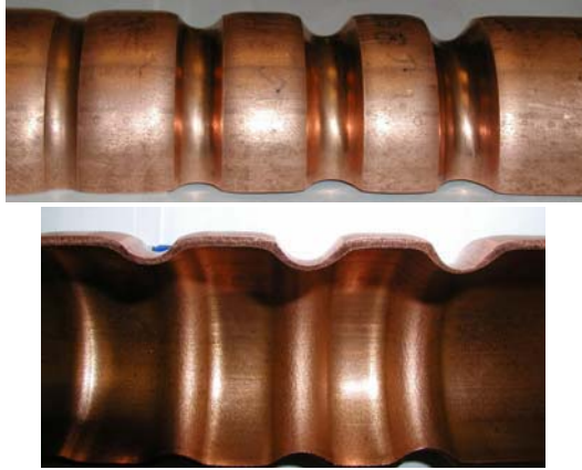
Figure 6: Samples of swaging or grooving of Cu tubes.
