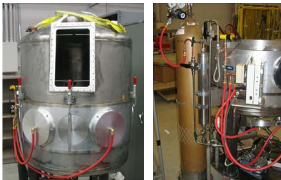
Figure 2: Chamber for high-purity TIG welding.
