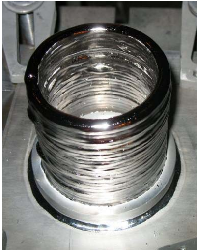
Figure 8: Niobium tube fabricated on polycrystalline substrate from wire using EBFFF.
