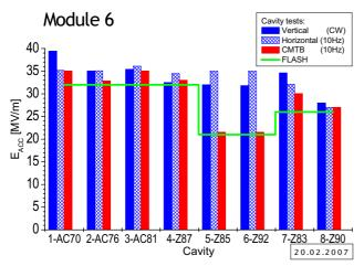
Figure 4: New FLASH SRF module 6 gradients.
