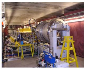
Figure 2: FLASH LINAC SRF module on the CMTB.
