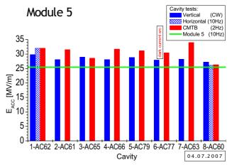
Figure 6: Repaired FLASH SRF module 5 gradients.
