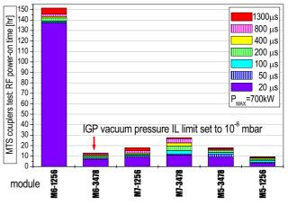
Figure 3: RF power rising time for different pulse lengths during the couplers conditioning on the CMTB.
