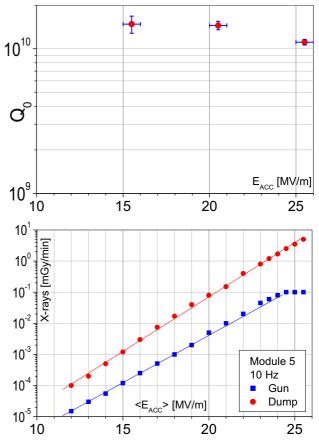
Figure 10: Repaired FLASH module 5 (ACC5) test results.
