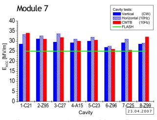
Figure 5: New FLASH SRF module 7 gradients.
