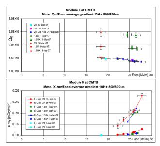
Figure 8: New FLASH module 6 (ACC6) test results.
